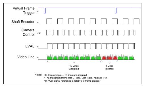
Figure 18: Synchronization Signals for a 10 Line Virtual Frame
