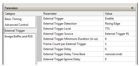
The Sync Master Xtium board is also configured to output the external trigger on board sync #1, as shown in the following image.
