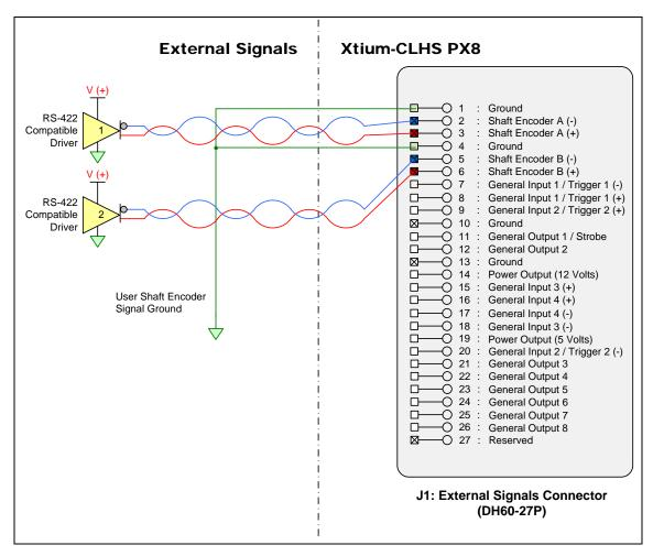
Figure 30:External RS-422 Signals Connection Diagram
