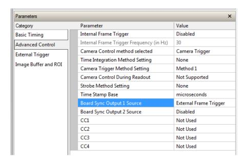
The Sync Slave Xtium board is configured to receive its trigger on the board sync signal. As an example the following image shows the Xtium board configured for an external sync on board sync #2.
