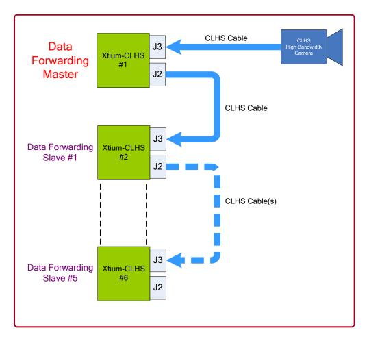
Figure 22: Data Forwarding Block Diagram
