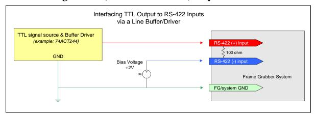
Figure 31: Interfacing TTL to RS-422 Shaft Encoder Inputs
