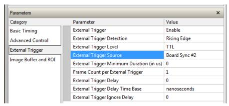
• **Test Setup:** Start the acquisition on all slave boards. The acquisition process is now waiting for the control signal from the master board. Trigger master board acquisition and the acquisition start signal is sent to each slave board.
