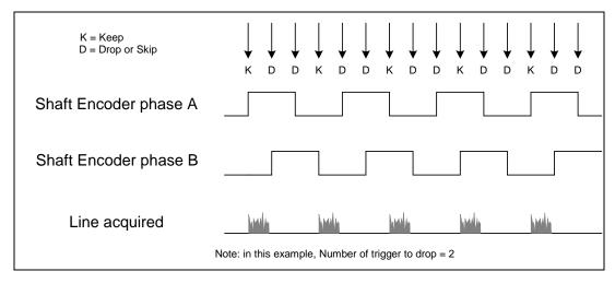
Figure 16: Encoder Input with Pulse-drop Counter
