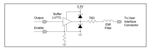
Figure 27: General Outputs Electrical Diagram
