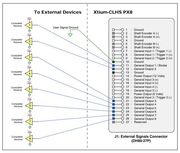
Figure 28:Output Signals Connection Diagram
