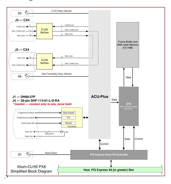
Figure 13: Xtium-CLHS PX8 Block Diagram
