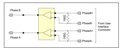
Figure 29: RS-422 Shaft Encoder Input Electrical Diagram
