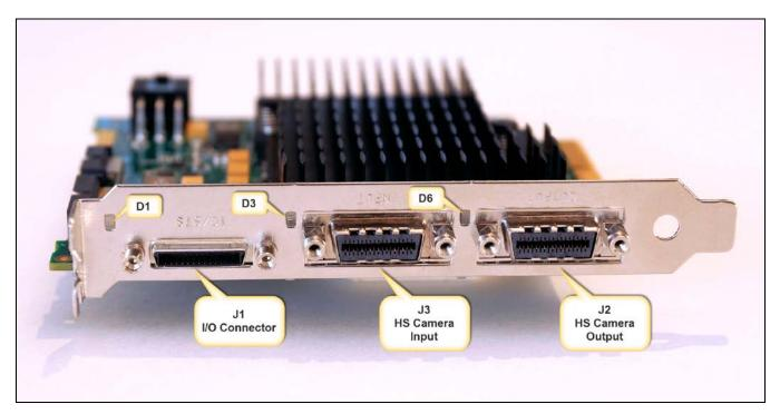
Figure 21: End Bracket Details
