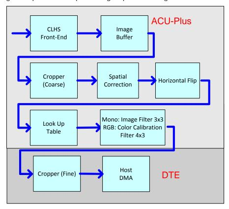
Figure 14: Xtium-CLHS Flow Diagram
