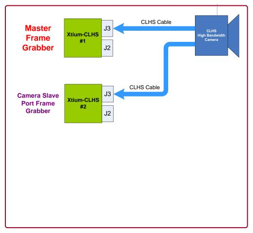
Figure 23: Dual Camera Output Connection Block Diagram
