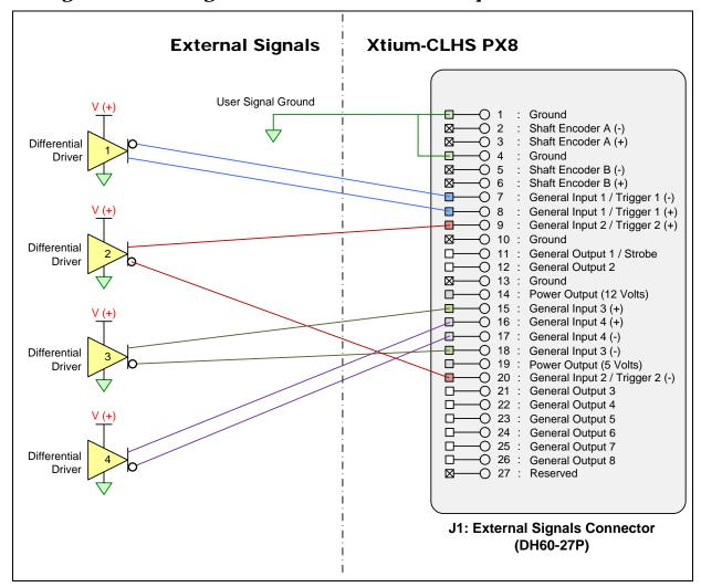
Figure 26:External Signals Connection Diagram
